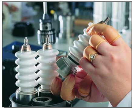
Metalization application and assembly process
