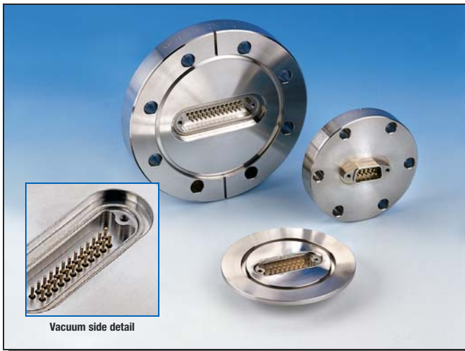
Type-D subminiature feedthroughs: 9-Pin on 2-3/4" Del-Seal™ CF flange, 15-Pin on ISO NW50 Kwik-Flange™, and 25-Pin on 4-1/2" Del-Seal™ CF flange. Air-side connector with snap on housing included, not shown above.
